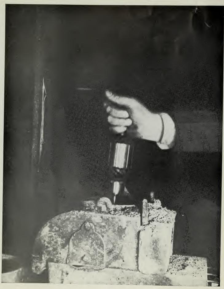
Solder flux is painted around the commutator where the wires have been tapped into the slots. The whole commutator is then immersed into solder, as shown above, the solder only adhering to the band where the flux has been applied.
